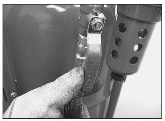
Figure 13. Blast nozzle air supply valve, opened.
